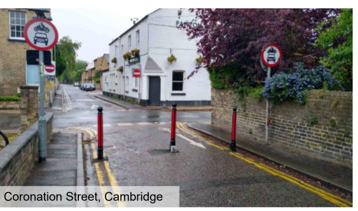
The use of modal filtering is absolutely key to unravelling the motoring and cycling networks.
