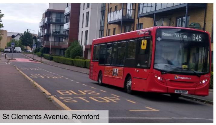
Here on a residential connector street, a bus gate to allow buses to serve the heart of a residential area, but which keeps through traffic out.
