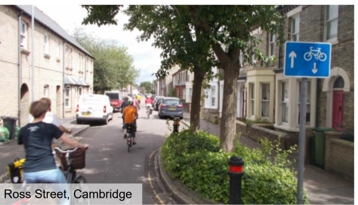
Working with narrower historic streets using one-way motor traffic loops, but with two-way cycling throughout.
