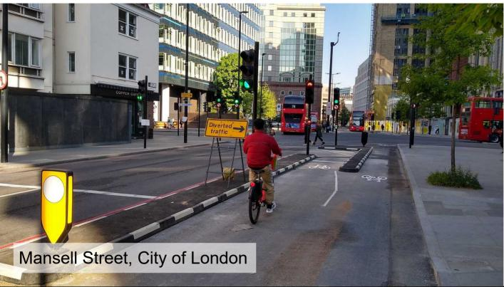
Offside cycle gate from a two-way cycle track with an oncoming movement.
