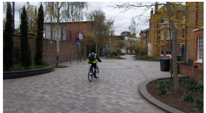
Van Gough Walk, Lambeth. Bespoke kerb units creating planting beds for a low speed limited vehicle access street.
