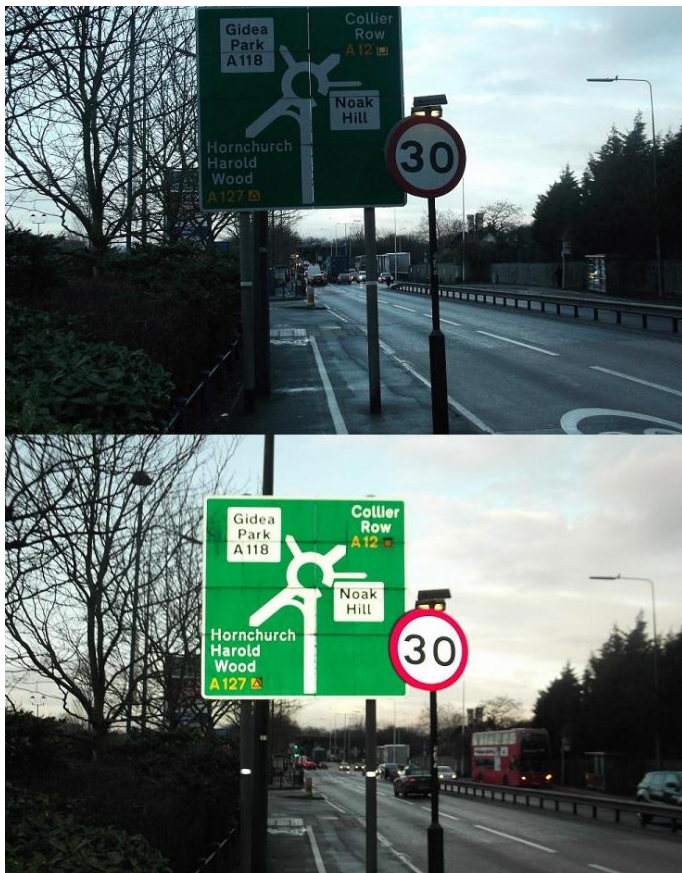
The upper photograph was taken without a flash and the lower photograph was taken with a flash to show retroreflectivity.
