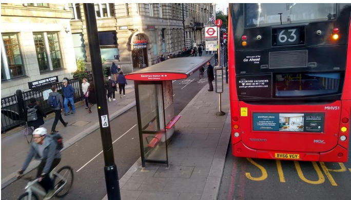
The floating passenger area here is not particularly wide and shelter proximity to the cycle track both creates a risk to people cycling clipping it and obscures the views between passenger and people cycling.
