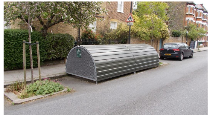
Secure on-street cycle parking. Curved cover opens for those with access and cycles are also locked onto internal hoops.
