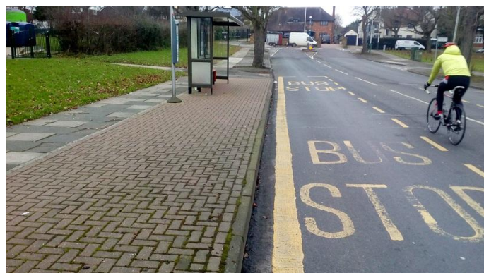
An accessible bus stop with a shelter that doesn't block the footway for people passing by.
