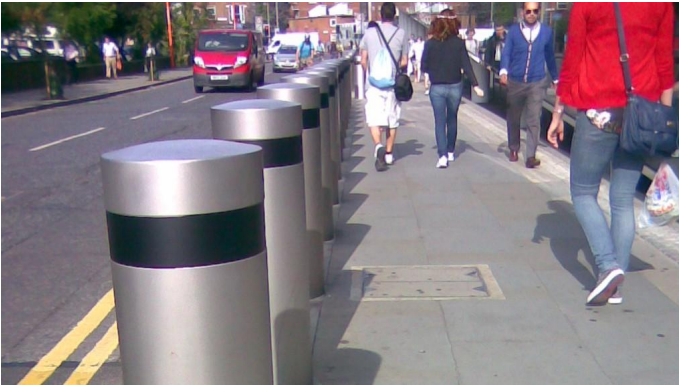
Bollards providing protection to an adjacent building which significantly reduce the available footway width.
